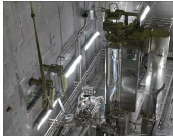
System for assembling fuel rods into the final fuel assembly structure
