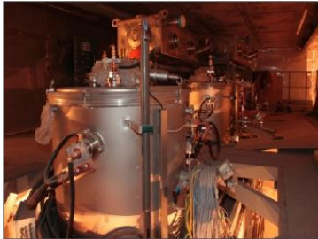
System for fuel pellets sintering, MOX fuel fabrication
