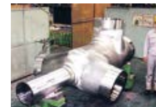
Primary Loop Piping
