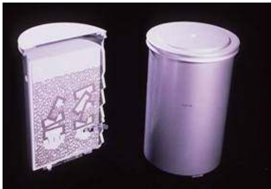
Structural materials in concrete matrix (before 1995)
