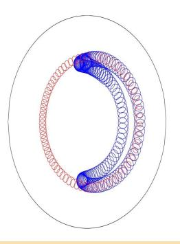
Projected particle orbits Charged Particles stay inside plasma
