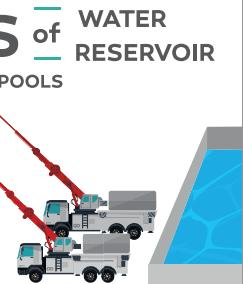
A reservoir has been built to store 20,000 tons of water 45m above sea level to inject fresh water into the reactors in case pumps cannot be used. Water cannon trucks have also been deployed to inject water into spent fuel pools at higher areas.
