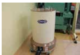
Compact NDA system incorporating a helium-3 substitute ceramic scintillator developed by
