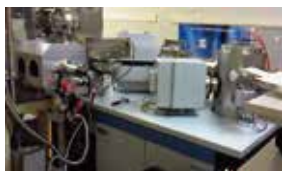
Surface ionization mass spectrometer for use in nuclear forensics
