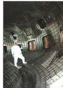
Inside of Vacuum Vessel About ten thousand carbon tiles protect the vacuum vessel from the high temperature plasma. In 1997, the divertor geometry at the bottom of the vacuum vessel was modified, in order to improve the heat and particle flux controllabilities.
