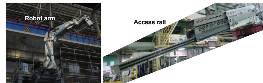
Figure 5: In-pedestal access device test
