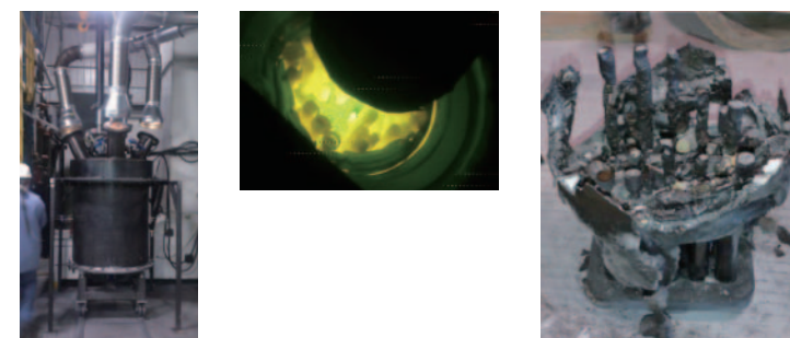
Figure 2: Simulated fuel assemblies plasma heating test (preliminary test device, heating condition, and tested unit)
