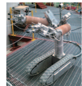
Figure 6: Prototype of flexible structure arm for remote operation
