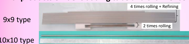
Fuel cladding tube of FeCrAl-ODS stainless steel (Length:>1m, Thickness:0.35mm)
