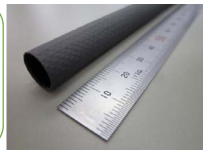
SiC fiber /SiC matrix composite (Trial product of fuel cladding tube)
