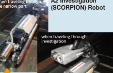
Scope of Investigation: Confirming conditions status of platform on the inside of pedestal in the PCV of Unit 2 Place of Investigation: Platform on the inside of the pedestal in the PCV of Unit 2 Development by: Toshiba Demonstration Testing Schedule: Second half of FY 2016
