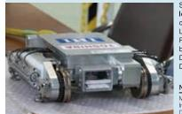
cope of Investigation: Adhering to outer surface of vent pipe to investigate eaks from the vent pipe-D/W joint and water flow inside a lower part of ncrete wall opening using lights and camera by remotely operation ocation of Investigation: Joint section of vent pipe in the torus room and CV shell (in the air) (schedule for actual use of robots in tasks has not yet velopment by: Toshiba
