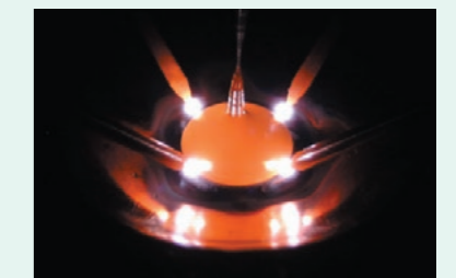
Single crystal sample grown by Czochralski process
