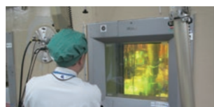
Analysis conducted in shielded cell (hot cell) by remote handling.
