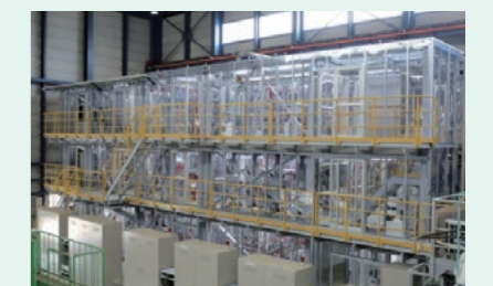
Continuous hydrogen production test facility made of industrial materials H 2 production rate: up to 0.1m 3 /h-H 2 Size: W18.5×D5×H8.1 (m)
