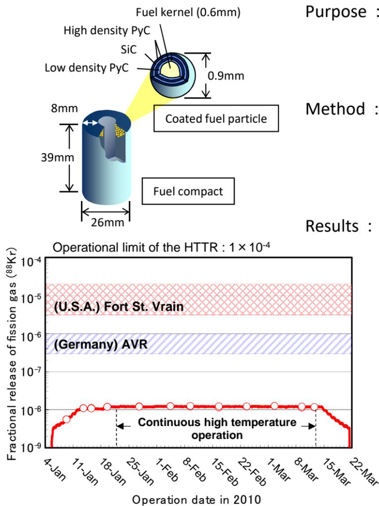
**Purpose :** High temperature strength of the ceramics coating layers to retain fission products inside the coated fuel particle
