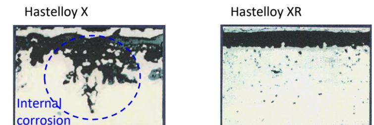
Cross-section photo after 1000°C 10000hr corrosion test
