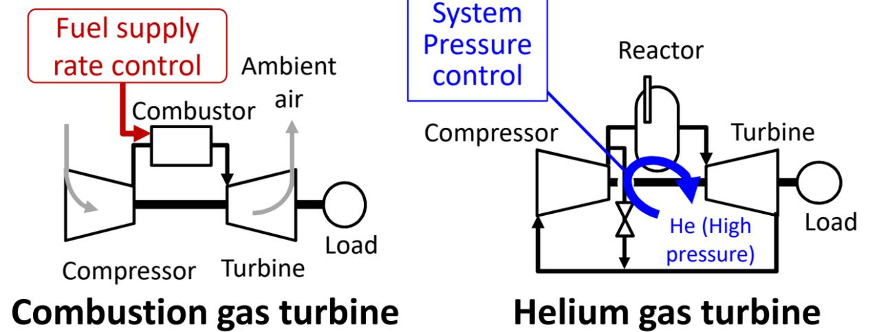
A method for stable operation by system pressure control should be established
