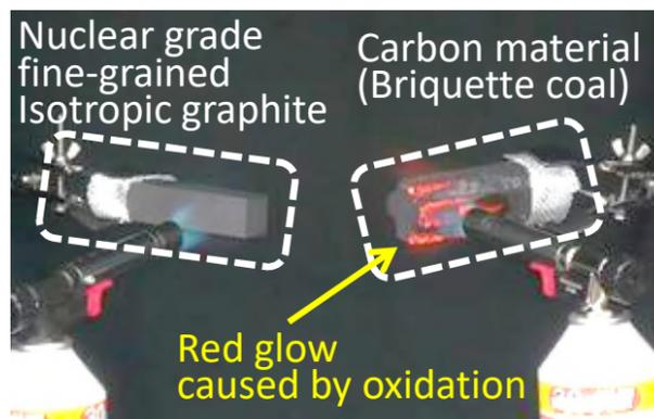
Appearance of nuclear grade fine-grained isotropic graphite and carbon material during burner heating
