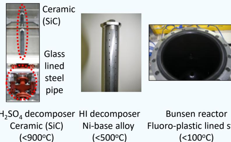
Verification of integrity of key components in the IS process environment (corrosion resistance, heat resistance)
