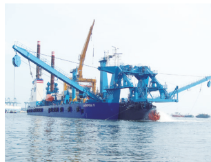
"CASSIOPEIA V" Self-Propelled Cutter Suction Dredger with Cutting-edge Technology
