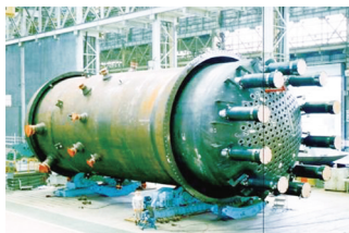
Reactor Pressure Vessel (ABWR)
