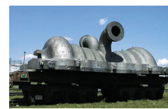
Steam Turbine Casing
