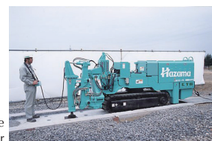
Compaction Machine for LLW Bentonite Barrier
