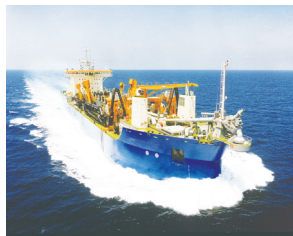
"ANDROMEDA V" Trailing Suction Hopper Dredger for Mega Scale Reclamation Works
