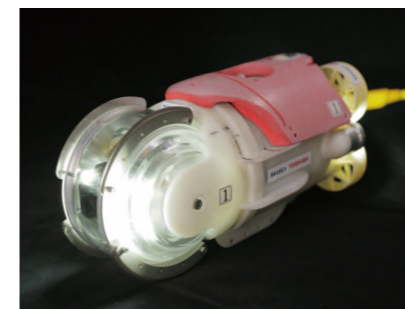
Unit 3 investigation robot
