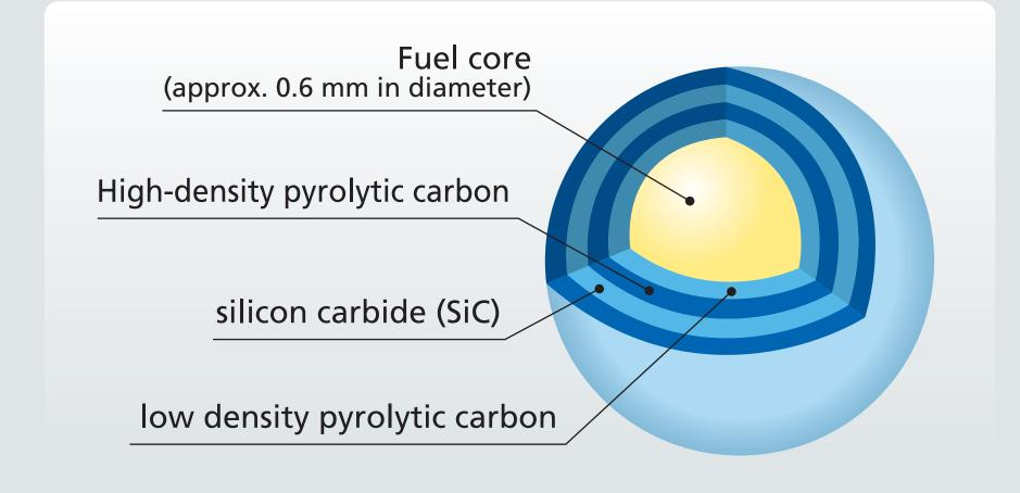
Extremely difficult to melt fuel because of the rigid (four-layer) coating of the fuel
