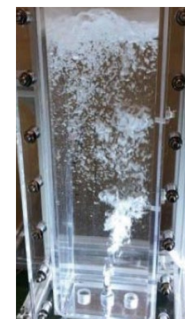
▲ Testing particle migration at the gas-liquid boundary (Figure 14)
