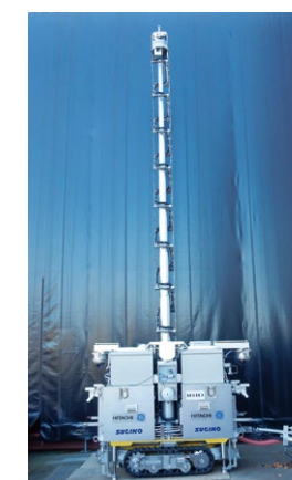
▲ High-pressure water jet decontamination equipment for high places (Figure 5)
