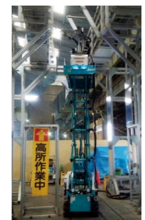
▲ Dry-ice blast decontamination equipment for high places (Figure 6)
