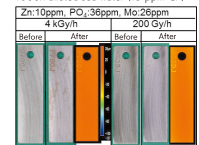
▲ Testing the effectiveness of the corrosion inhibitor under \gamma radiation (Figure 3)
