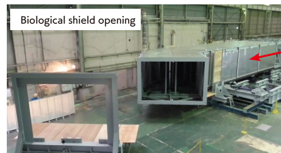
▲ Element testing for delivery of the access tunnel
