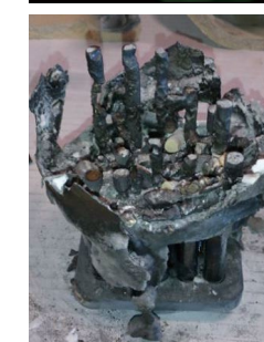
▲ Plasma-heating test on simulated fuel assembly (during heating and the test piece after)
