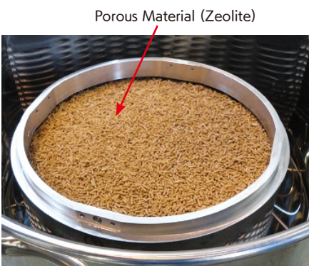
▲ Test piece in drying test (Figure 10) Drying tests were conducted using zeolite, a porous material.
