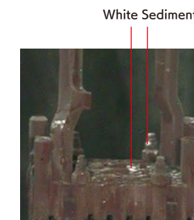
◀ Results of visual inspection of spent fuel from Unit 4 (upper tie plate of fuel mixed with rubbles) (Figure 2)
