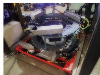
▲ Positioning system for extension pipe (Figure 6)
