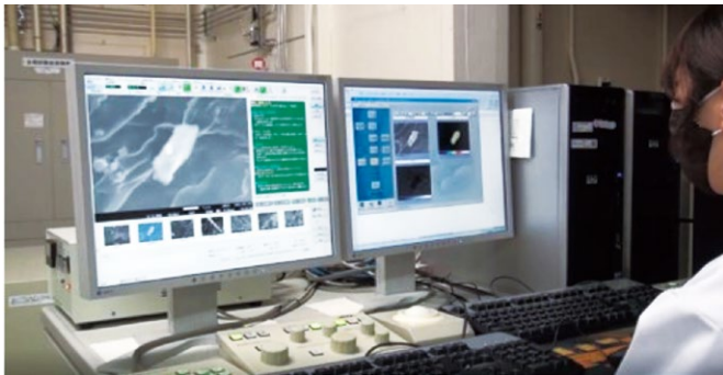
▲ Conducting a SEM* analysis on the sample of accreted material collected inside the reactor (Figure 16) At the JAEA Oarai Research and Development Institute *SEM: scanning electron microscope
