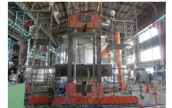
▲ Testing the durability of the RPV pedestal (miniaturized testing equipment) (Figure 4)
