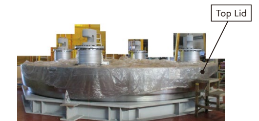
▲ Testing the top lid of a dedicated (large) transport container
