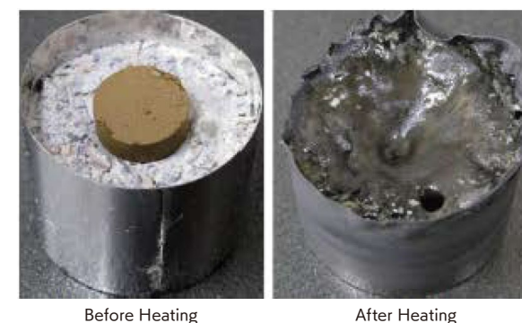
▲ Creating simulated MCCI product via condensed-light heating (Figure 1)
