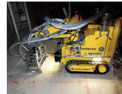
▲ High-pressure water jet decontamination equipment (Figure 2)
