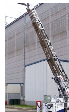
▲ Suction and blast decontamination equipment for high places (Figure 4)
