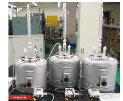
▲ Conducting the long-term corrosion test (Figure 5)
