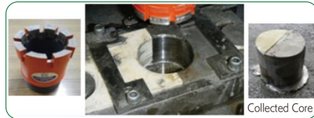
▲ Core boring; accumulation of water fine debris powder and in the cored hole
