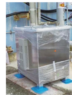
▲ Small muon-transmission measuring equipment (Photo 2) (Dimensions: approx. 1 m × 1 m × 1.3 m [height])
