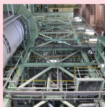
Large Scale Test Facility (Thermal-hydraulic integral effects test facility for PWR) LSTF
