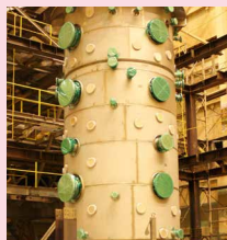
Containment Integral Measurement Apparatus CIGMA
