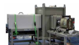
Delayed gamma-ray analysis instrument, tested at the JRC Ispra (Italy)
