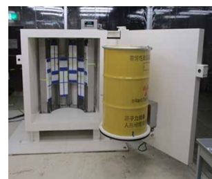
Complex shape-supporting clearance level testing apparatus
