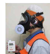
Heat stroke monitoring and warning device
