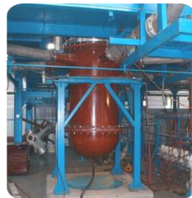
Mixing Tests of reactor vessel down-comer
