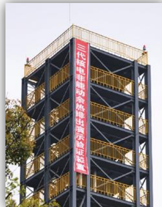
Passive residual heat removal test for secondary side
