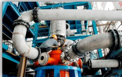
Flow-induced Vibration Simulation Test of Reactor Internals
