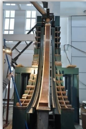
Test of Cavity Injection and Cooling System
