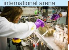
Platform of mixers and settlers to validate the performance of the selective uranium extraction process on a laboratory scale
