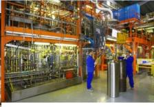
General view of the evolving vitrification prototype equipped with a cold crucible melter adapted for nuclear environments at Marcoule
